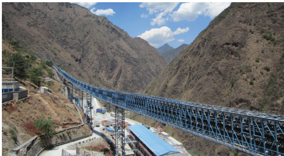
A conveyor belt removes rock from JinPing laboratory, a 2,500-metre-deep dark-matter experiment site.
